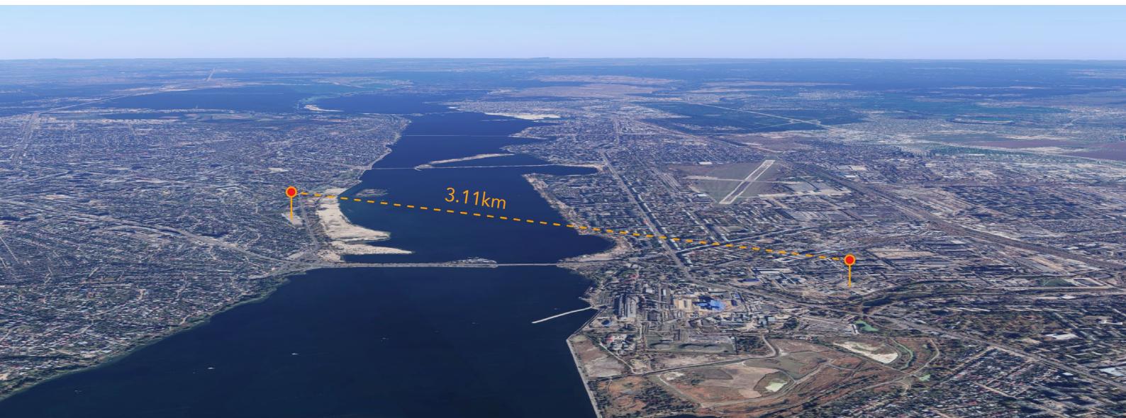
Map | LigoDLB 6ac Link with External Dish Antenna (3.11km)
